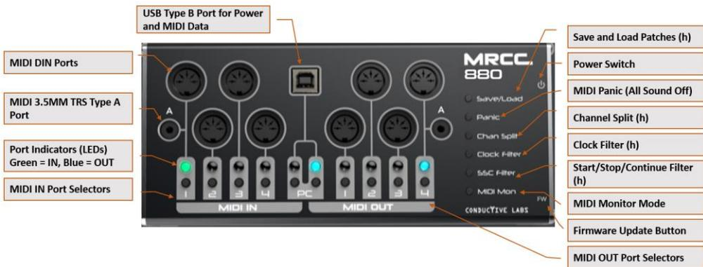
(h) = Press and hold the button while selecting an input port to apply the filter to. MRCC 880 will blink the LEDs to indicate appropriate port choices.
