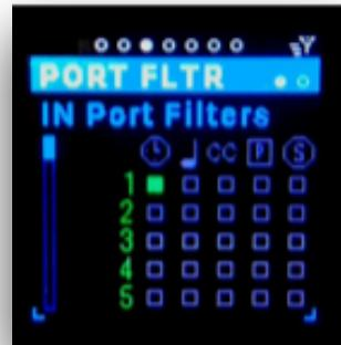
Use the UP and DOWN buttons to select the scrollbar, the port number or a filter, use the encoder to select a row (via the scrollbar), a port number, or toggle a filter on or off for that port.
