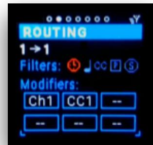
The current routing is also indicated by the routing LEDs, in cases where one input is routed to several outputs, the LED representing the output for the current routing is brighter than the others. You can select another routing to edit by pressing the ROUTING BUTTONS, or even create a new routing without leaving the routing screen.
