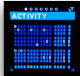
**Rows** (top to bottom): 6x DIN/TRS inputs inputs (2 rows of 3), 4x USB host inputs, and the USB PC port on the bottom.
